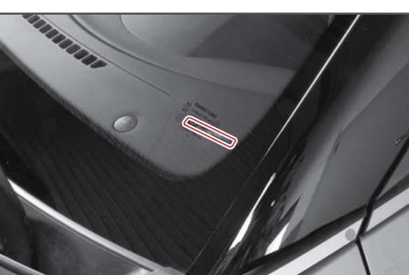
Visual VIN label is located on the driver's side instrument panel.
