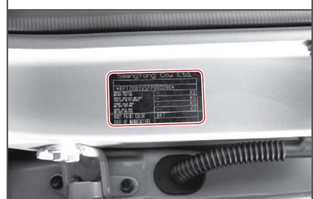
The certification label is located on the driver's door sill.
